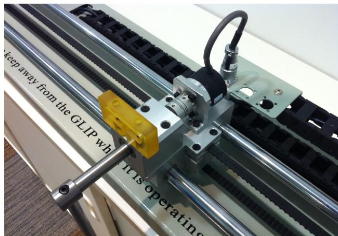
Figura 3.4: Network controled inverted pendulum
