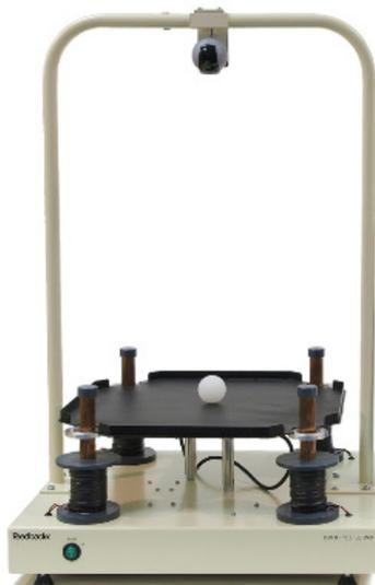
Figura 3.2: Ball and Plate Control System
