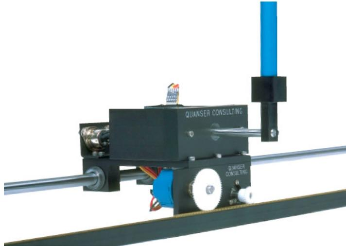
Figura 3.3: Self erected inverted pendulum
